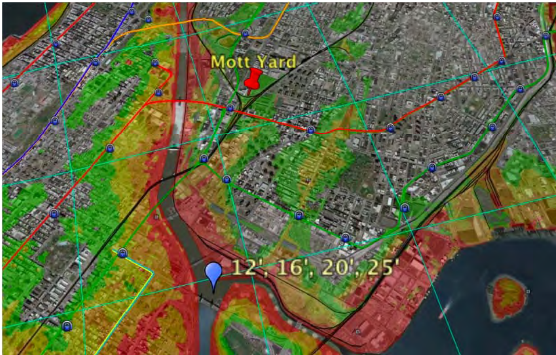
Figure 14: Location of the Mott Yard, Bronx, at the Y-shaped branching of the Metro North Lines. The Hudson Line takes the NW branch, and the Harlem/New Haven Lines take the NE branch of the 'Y' pattern of tracks (in gray). Note their combined SW crossing of the Harlem River into Manhattan to continue into Grand Central Station. Also shown is the relation to storm surge flood zones for worst-case tracks of hurricanes with different Saffir-Simpson (SS) categories. SS1 flood zone in red, SS2 in brown, SS3 in yellow, and SS4 in green. The blue grid defines the cells for the SLOSH computations for which the storm surge heights were calculated by the US Army Corps of Engineers / National Weather Service. At the location of the blue symbol, the approximate SLOSH worst-track storm surge heights are indicated; for SS1 about 12 feet; SS2 about 16 ft; for SS3 about 20 ft; for SS4 about 25 ft. Note that the likelihood of an intense worst-track hurricane is very low. See text for details.
