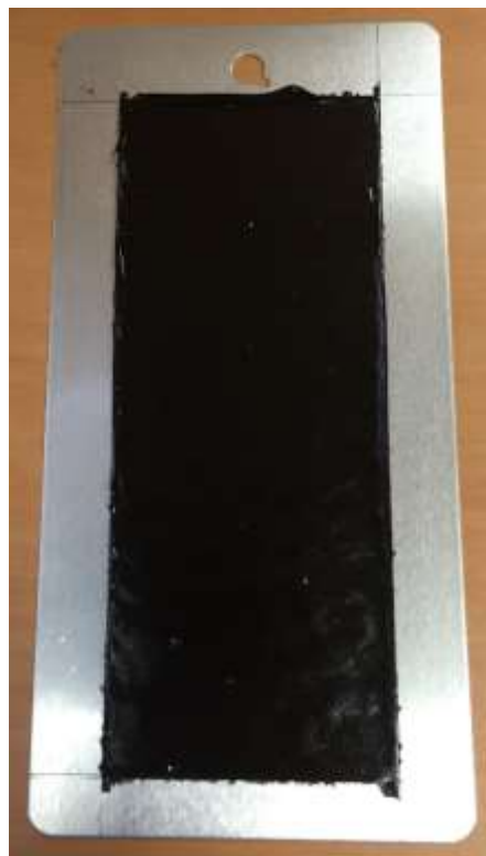
Figure 5: Asphalt Specimen after Masking Tape is Removed
