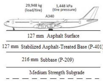
Laboratory-compacted specimens of each modified asphalt mixture were tested using AASHTO standards to determine volumetric properties and mechanical responses. The effects of static and dynamic aircraft loading were evaluated in ABAQUS™ using the material properties of the mixtures
