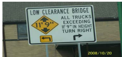
Figure 3-1: Low Vertical Under-clearance Sign Installed near the Bridge on George Urban Blvd in the Village of Depew, New York.
