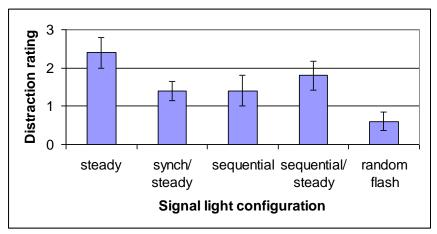
Figure 4-10. Mean distraction ratings (+/- standard error of the mean) for the configurations in the second evaluation set.
