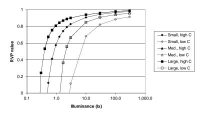
Figure 2-6. RVP values for a combination of task sizes and contrasts, for a 40-year-old worker, with glare of 2 lx present.
