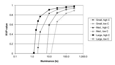
Figure 2-10. RVP values for a combination of task sizes and contrasts, for a 60-year-old worker, with glare of 20 lx present.
