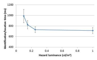
*Figure 3-7. Mean (+/- s.e.m.) identification times for the hazard detection experiment.*
