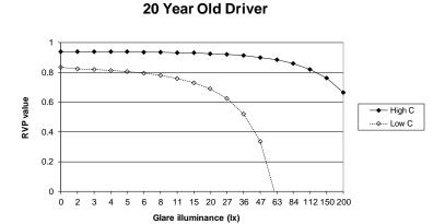
Figure 2-11. RVP values for high- and low-contrast targets viewed by 20-year-old drivers, as a function of the glare illuminance.
