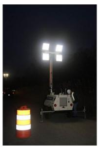
Figure 2-18. Light tower with four 270 W LED lights.
