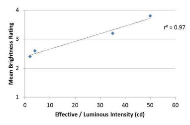
Figure 4-12. Relationship between barricade light intensity and perceived brightness.
