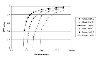
Figure 2-7. RVP values for a combination of task sizes and contrasts, for a 60-year-old worker, with glare of 2 lx present.
