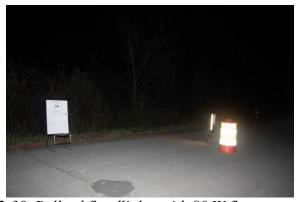
Figure 2-30. Bollard floodlights with 80 W fluorescent source.
