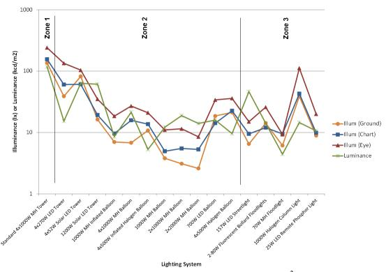
Figure 2-35. Measured light levels (in lx for illuminance, in  $kcd/m^2$  for luminance) for each system. Also shown are the zones for each lighting system.
