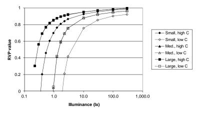
Figure 2-5. RVP values for a combination of task sizes and contrasts, for a 20-year-old worker, with glare of 2 lx present.
