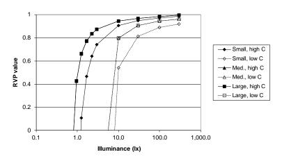
Figure 2-8. RVP values for a combination of task sizes and contrasts, for a 20-year-old worker, with glare of 20 lx present.
