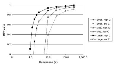
Figure 2-9. RVP values for a combination of task sizes and contrasts, for a 40-year-old worker, with glare of 20 lx present.
