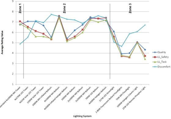
Figure 2-36. Average quality, light level (safety and task), usability and discomfort ratings for each lighting system. Also shown are the zones for each lighting system.
