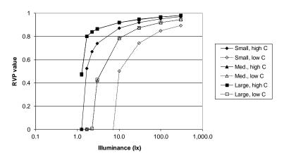
Figure 2-4. RVP values for a combination of task sizes and contrasts, for a 60-year-old worker.
