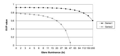
Figure 2-12. RVP values for high- and low-contrast targets viewed by 40-year-old drivers, as a function of the glare illuminance.
