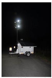
Figure 2-20. Solar-powered light tower with 1200 W LED lights.
