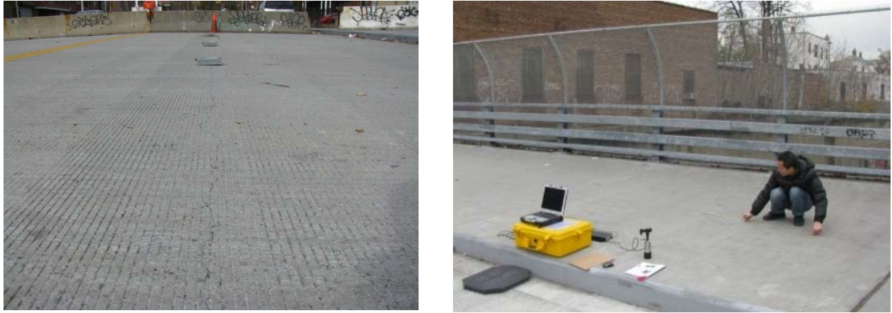
Fig. 4 Collect data manually using impact-echo on a bridge in Flushing, NYC
