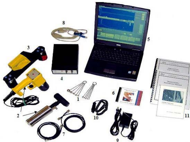
Fig. 5 a) Impact echo device from Impact Echo Instruments, LLC at Ithaca, New York, which is founded by Mary J. Sansalone in 1997. Item 1 is a set of 10 impactor, item 2 includes two hand-held transducers, item 3 is a dual-head transducer to measure the wave speed.
