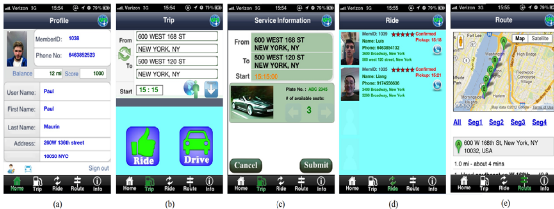
Figure 6 Interface of OMITS App on smart phones: (a) member management, (b) new service request (c) service information, (d) rider information for rider sharing, and (e) dynamic route direction and pick-up sites
