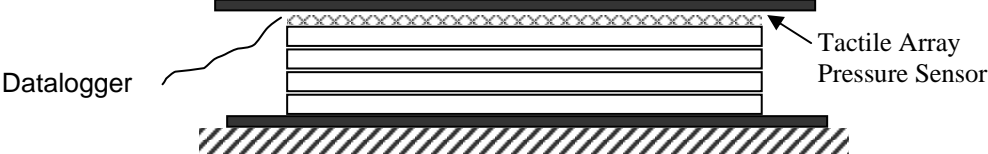
Figure 2.8. Bearing Instrumentation using Tactile Pressure Sensor
