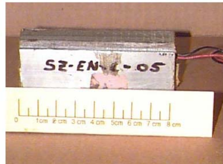
Photograph of the final sensor assembly ready for loading tests.
