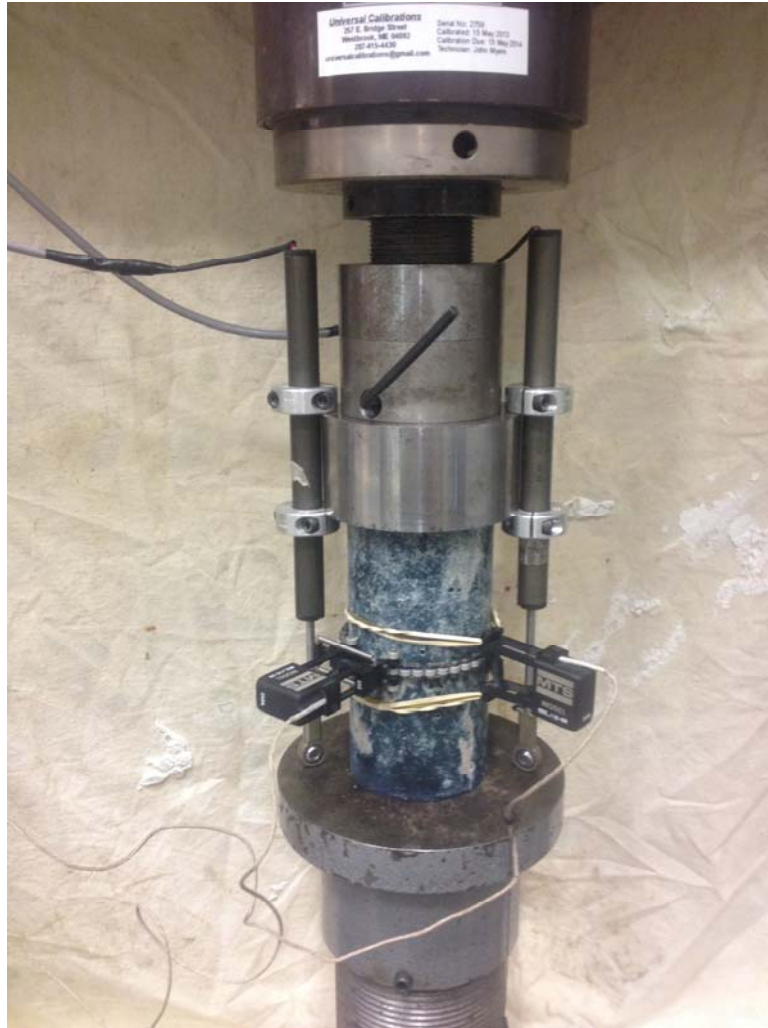
Figure 2: Engineering property test setup. Axial strain was measured using the axial extensometer and linear potentiometers as shown. Lateral strain was measured using the radial extensometer as shown.
