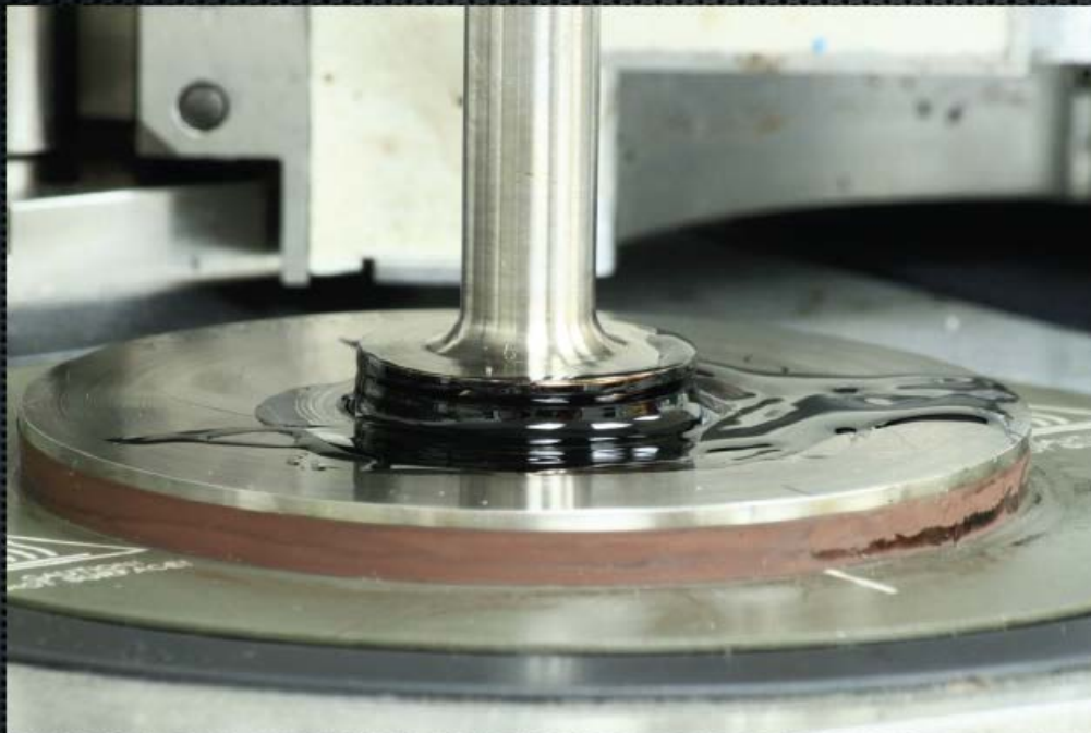
Figure 16 – 1.0mm Gap Height Immediately After Testing at 88°C
