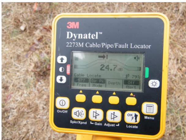
Figure 6: Trace wire receiver display shows an indication of signal level and wire location.
