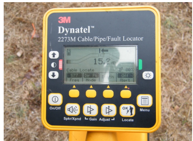
Figure 6: Trace wire receiver display shows an indication of signal level and wire location.
