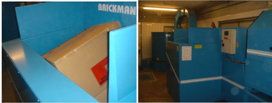
Figure 3-6. An OCC Brick Machine Connected to a Pneumatic Network (Source: Envac, 2011)
