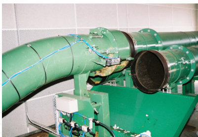
Figure 1-9. Three-Way Diverter Valve (Source: Kogler, 2007)
