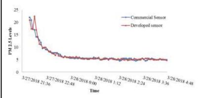
PM2.5 Comparison between Dylos and Developed Sensor
