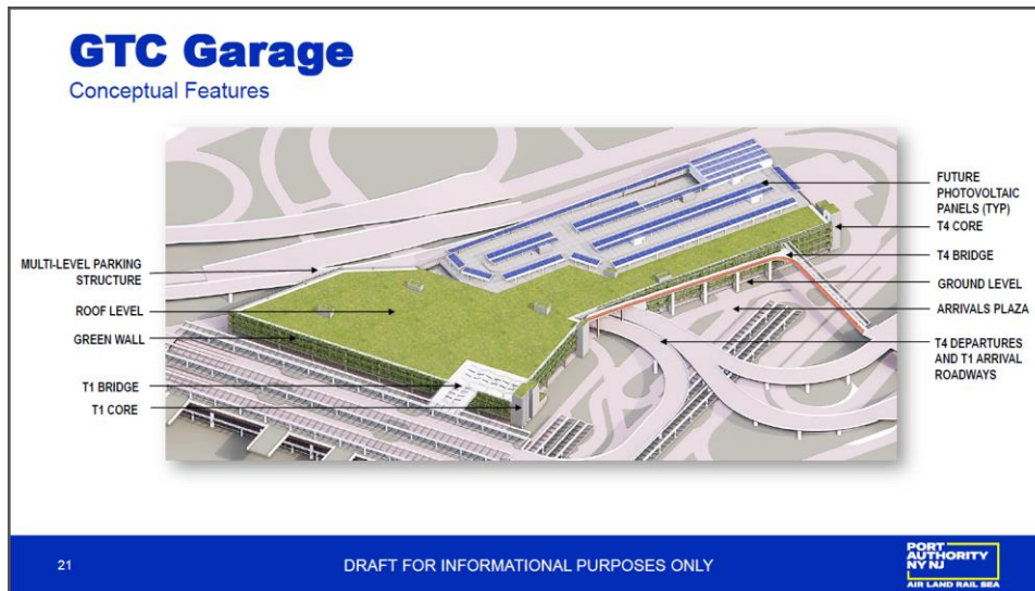
JFK Redevelopment Ground Transportation Center Garage. Image Credit: Port Authority NY & NJ
