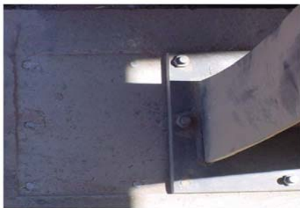
Failed Steel Column Connections in Explosive Tests
