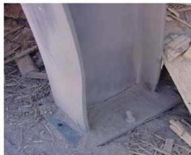
Failed Steel Column Connections in Explosive Tests
