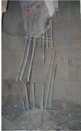
Figure 6.13: Severance of longitudinal rebar during a test by Matthews et al. (2007).
