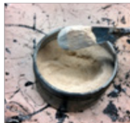
New Jersey dust used to make mastics (particles passing No. 200 sieve).
