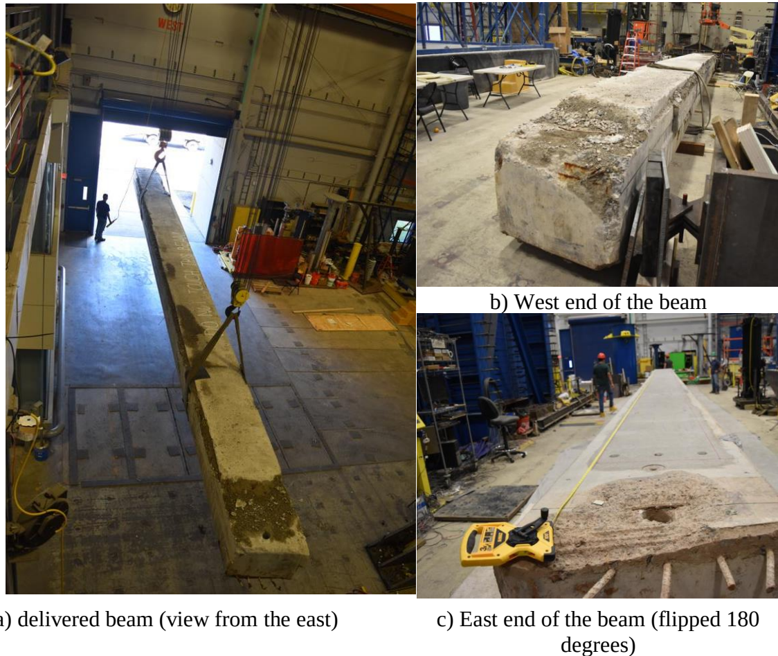
Figure 2-7 Overall condition of Beam 2 after delivery to the SEES laboratory
