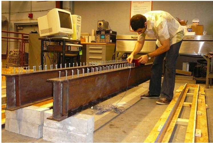
Figure 24. Installation of shear connectors and strain gauge instrumentation.
