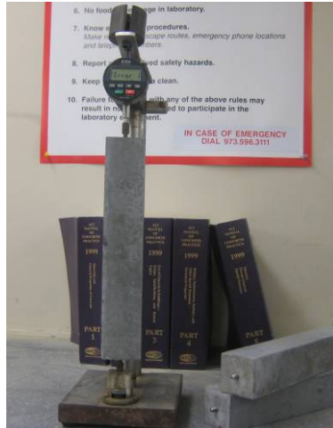
Figure A1. Measuring change in the length of a concrete shrinkage bars.
