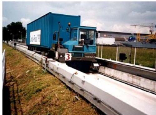
Figure 16. CombiRoad vehicle at the testing facility in Ridderkerk, Netherlands (courtesy of TNO)
