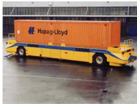
Figure 13. Kogel Kamag AGV for Port of Singapore (obtained from Kogel Kamag website)
