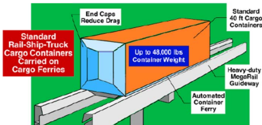
Figure 4. Schematic picture of the CargoRail "Freight Ferry" on the guideway (courtesy of MegaRail Transportation Systems, Inc.)
