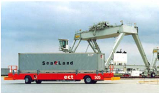
Figure 11. AGV operating in European Combined Terminal (ECT) in Rotterdam, Netherlands (obtained from Frog Systems website)
