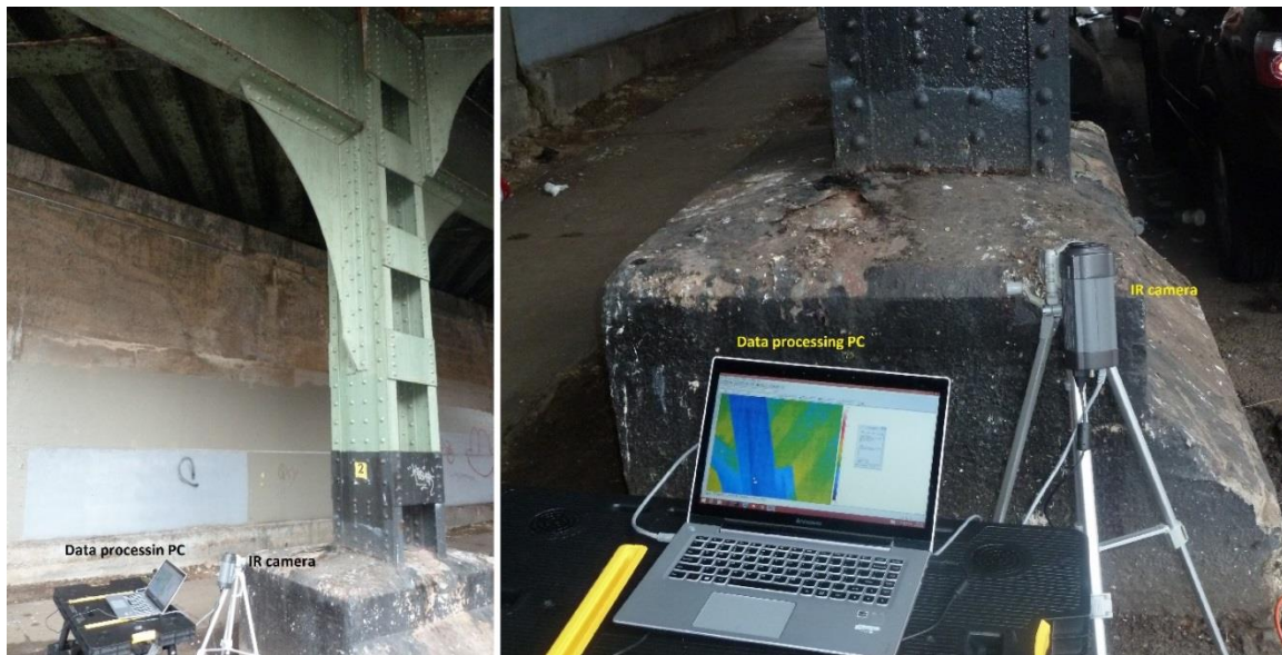
Figure 6. Equipment setup for thermography inspection of bridge steel beams
