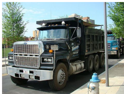
Type 7: Single unit trucks with > 3 axles
