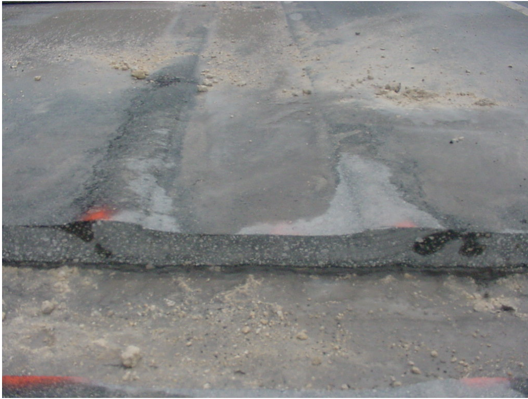
Figure B-4. Section 4-A showing no deformation of the base layer – Most of the deformation is due to instability in the asphalt concrete.
